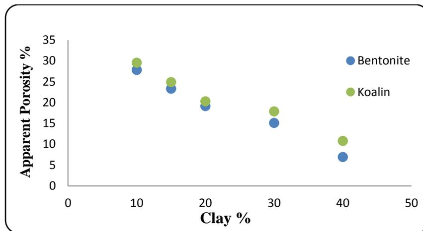
**Figure 3:** Apparent porosity for K-mortar and B-mortar.
