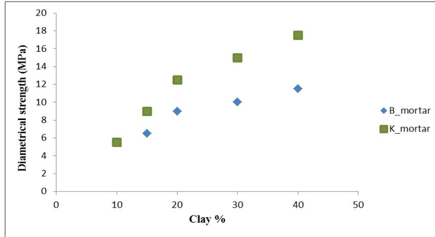
**Figure 5:** Diametric strength for K-mortar and B-mortar.
