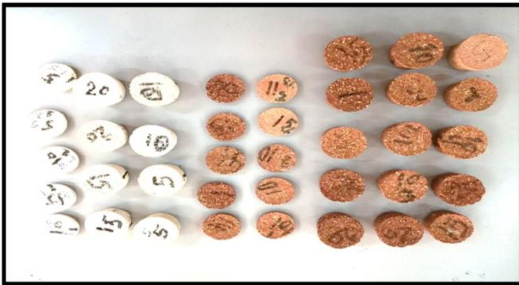
**Figure 1:** Specimen after firing at 1200 °C.
