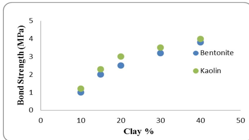
**Figure 4:** Bond strength for K-mortar and B-mortar.
