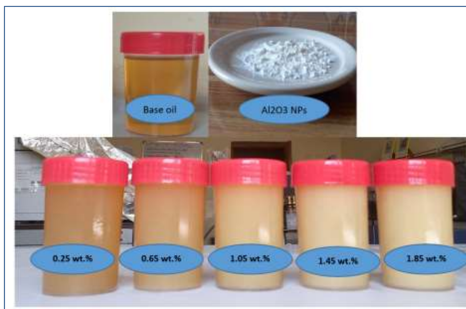
Figure 8: Testing nano-lubricants stability for 60 days at different Al 2 O 3 NPs additions.
