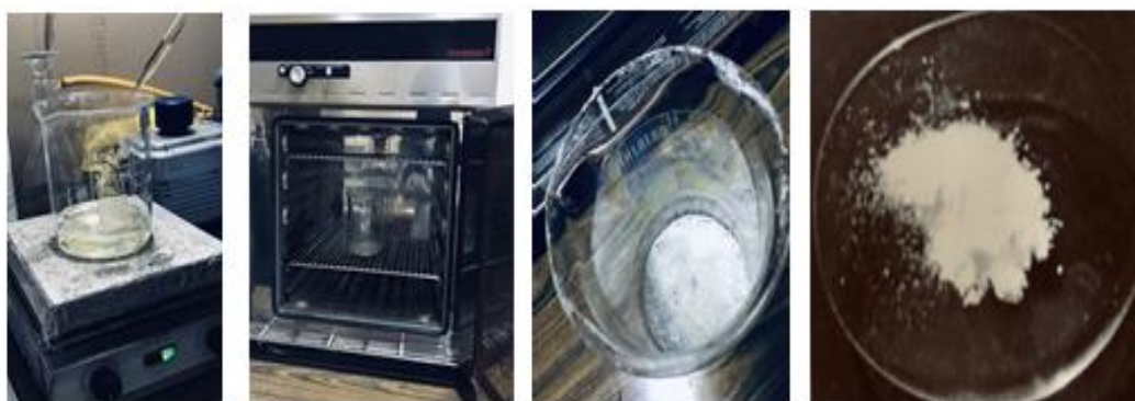
Figure 2: Steps of synthesis MgO using Sol-gel technique
