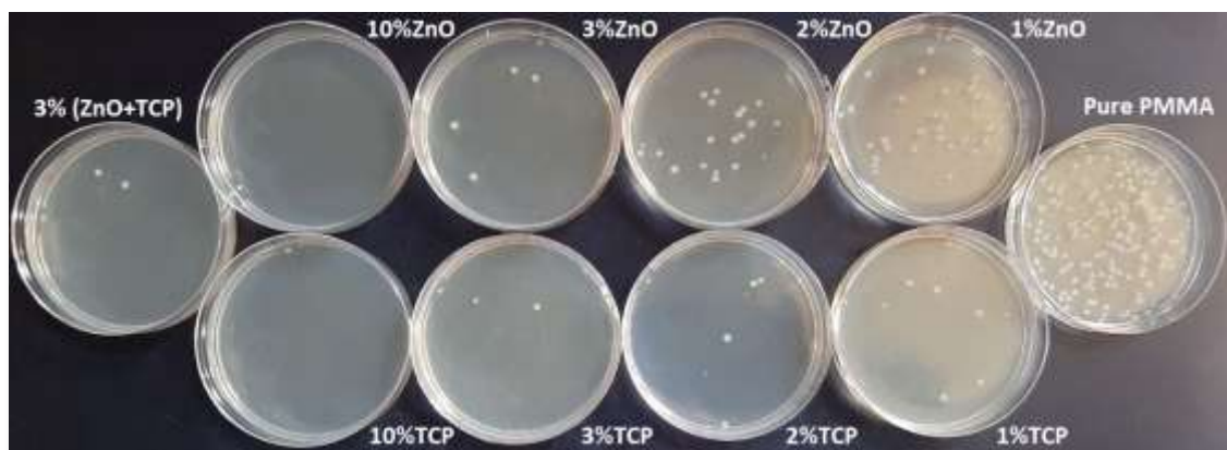
Figure 9: This graph illustrates a reduction in the number of S. aureus adhering colonies to the surfaces of samples reinforced with certain ratios of nanoparticles in comparison to a PMMA-free nanoparticles sample that has been used as a control.
