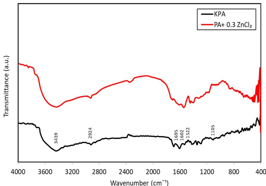
**Figure 3:** FTIR spectra of PAA and Zn-PA (0.3 g of  $\text{ZnCl}_2$ ).
