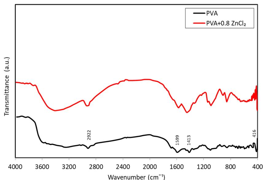
**Figure 4:** FTIR spectra of PVA and Zn-PVA (0.6 g of  $\text{ZnCl}_2$ ).
