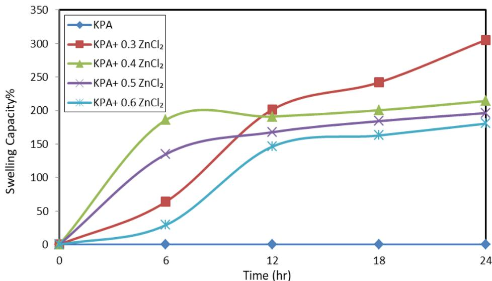
**Figure 8:** Swelling Ratio (%) of KPA and (Zn-KPA) SAPs.
