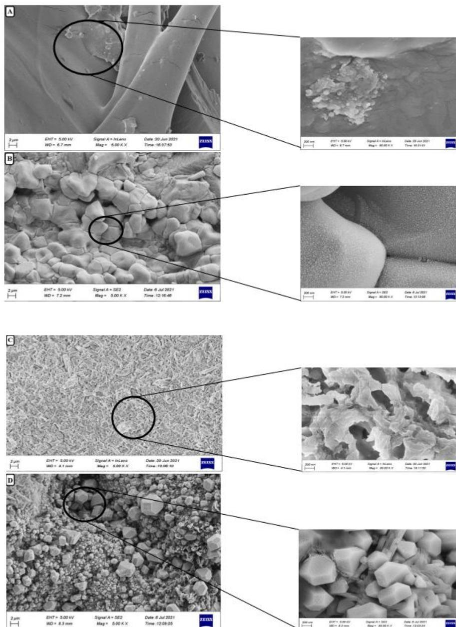
**Figure 7:** SEM micrographs of (A) KPA, (B) Zn-PA (0.3 g of ZnCl<sub>2</sub>) (C) PVA and (D) Zn-PVA (0.8 g of ZnCl<sub>2</sub>).
