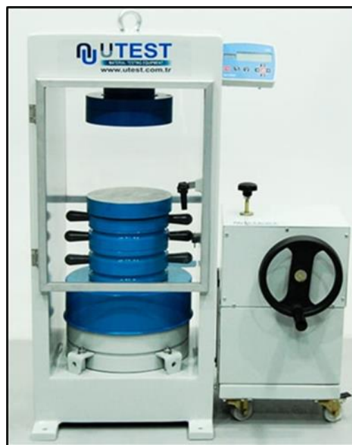
Figure 2: Compressive strength test machine.
