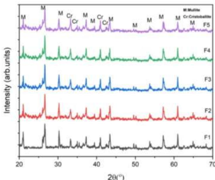
**Figure 2:** The XRD pattern of the prepared specimens.
