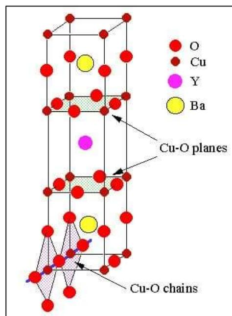
**Figure 5:** Part of the lattice structure of Y-Ba-Cu-O [44].
