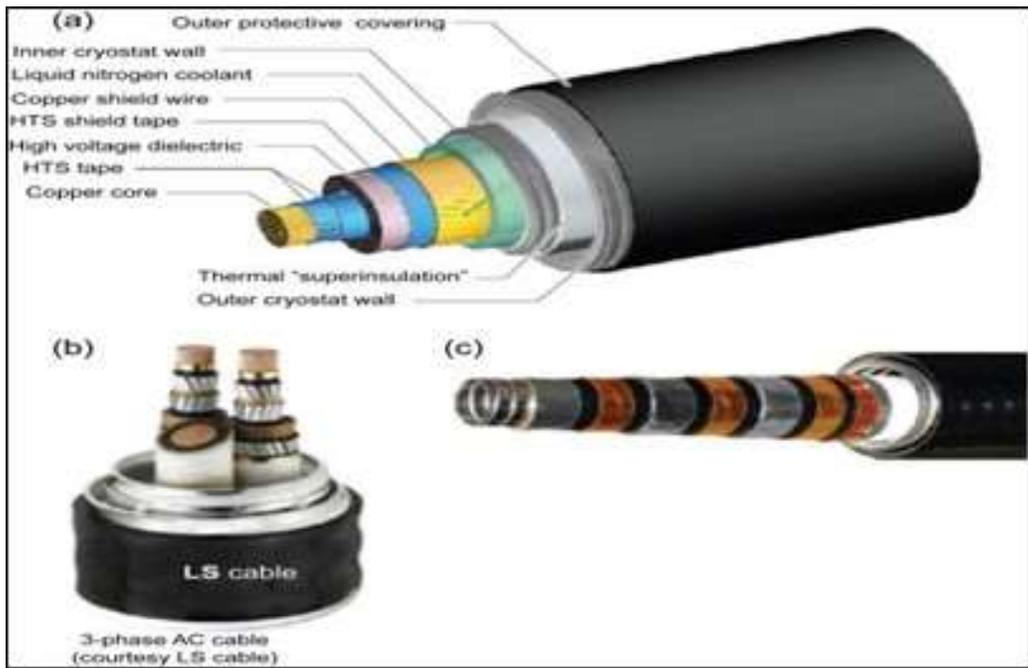
Figure 11: Typical HTS superconducting power transmission Cable Structure [90].
