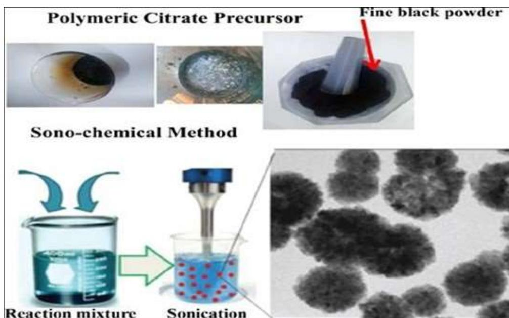
**Figure 7:** Illustration of Citrate Pyrolysis Technique [58].
