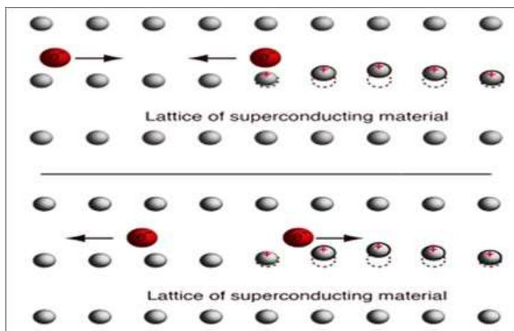
**Figure 3:** The generation of attractive force between electrons in a crystal. a) When an electron passes through the lattice, it attracts it and causes a little wave along its path. b) The displacement attracts another electron traveling in the opposite direction [19].
