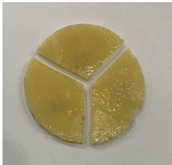
Figure 10: Broken specimen after pistons on three balls test.
