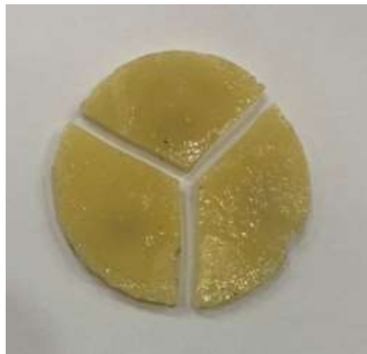
Figure 8: Broken specimen after pistons on three balls test.
