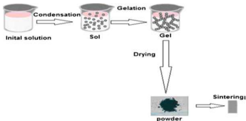
Figure 8: Schematic diagram of sol gel process for production nanopowders [65].
