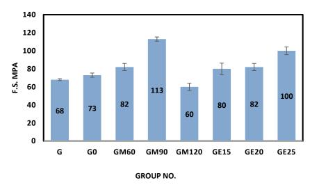
Figure 7: The flexural strength test values of denture base acrylic resin PMMA reinforced with scratched and anodized SS316L wires.
