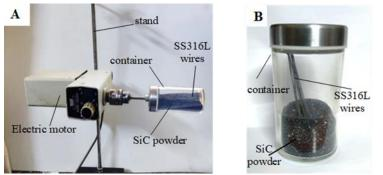
Figure 1: (A) system of mechanical treatment, (B) SS316L wires, and SiC powder in the scratching container.
