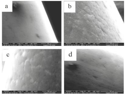
Figure 5: Scanning electron microscope images of untreated (a) and treated (b to d) scratched stainless steel 316L wire surfaces.
