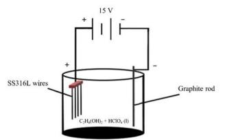
Figure 2: Show the anodizing system of Ethylene Glycol electrolyte with 5% Perchloric acid.
