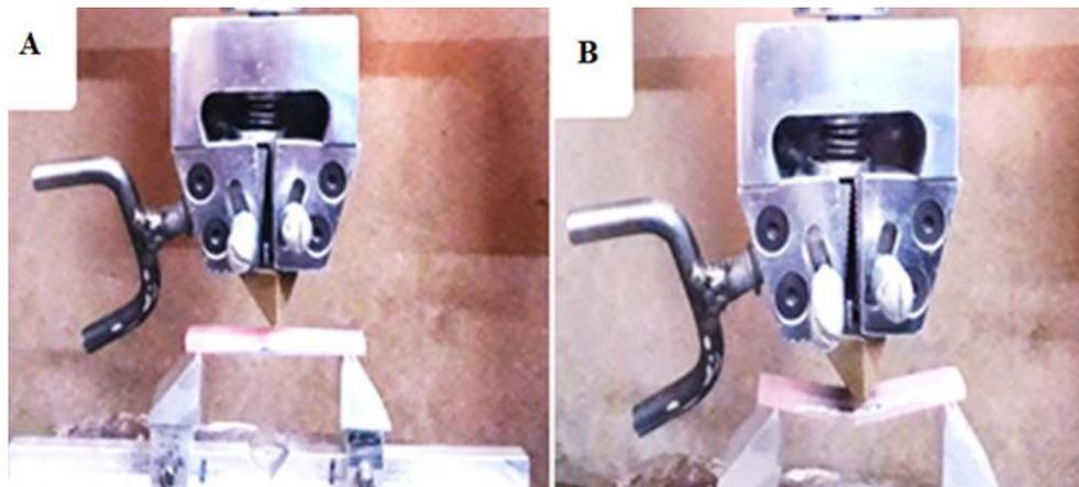
**Figure 4:** Flexural strength test instrument: A: The sample in test B: Sample after test.
