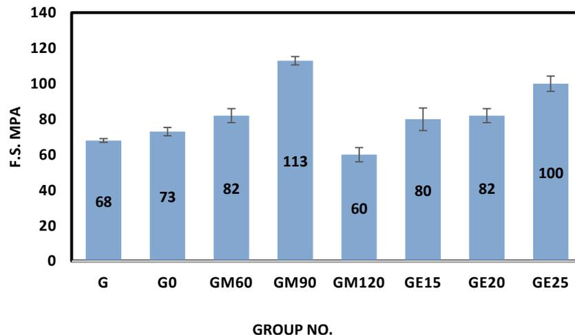
**Figure 7:** The flexural strength test values of denture base acrylic resin PMMA reinforced with scratched and anodized SS316L wires.
