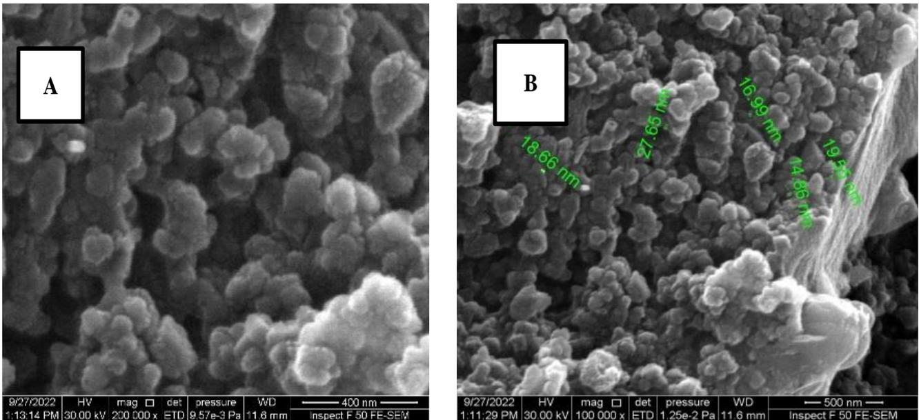
**Figure 10:** SEM picture of nanoparticles: A) First sample / C2, B) Second sample/ C4.
