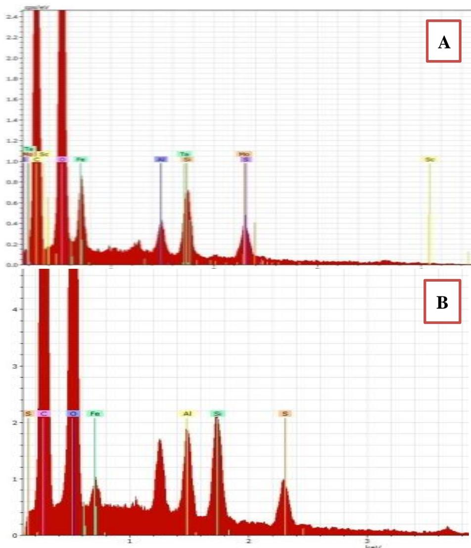
Figure 5: EDX-analysis before burning: A) First sample, B) Second sample.
