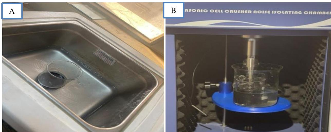
**Figure 4:** Ultrasound tools: A) ultrasound machine bath samples (C1 & C3), B) ultrasound machine probe samples (C2 & C4).
