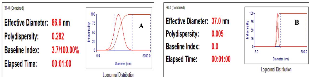
**Figure 7:** Partical size analyses for sonication bath samples: A) The first sample/ C1, B) The second sample/ C3.
