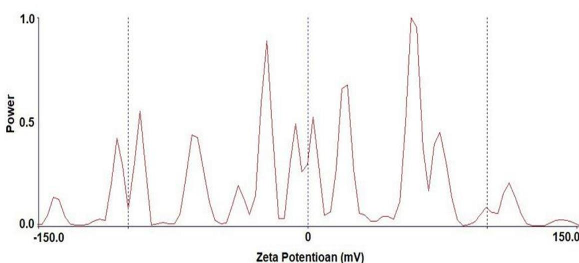
**Figure 11:** Zeta potential of prepared carbon nanoparticles.
