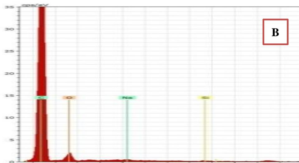
**Figure 6:** EDX-analysis after burning, Nano size: A) First sample, B) Second sample.
