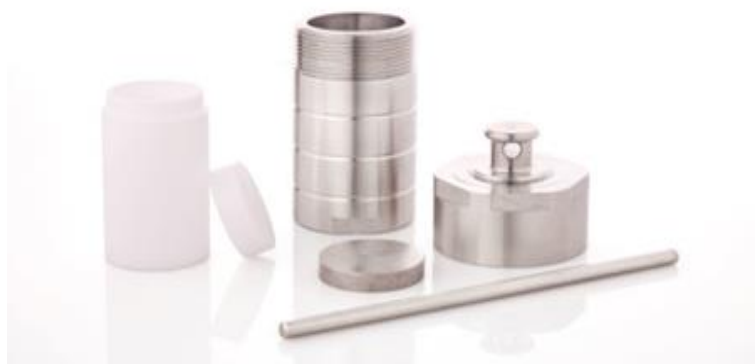
Figure 4: Image of Teflon lined stainless steel autoclave with inner components [37].
