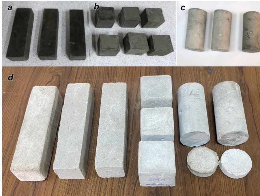
Figure 1: Different testing samples before and after setting. a- flexural strength samples, b-compressive strength samples, c-splitting tensile strength samples, and d- samples after setting.
