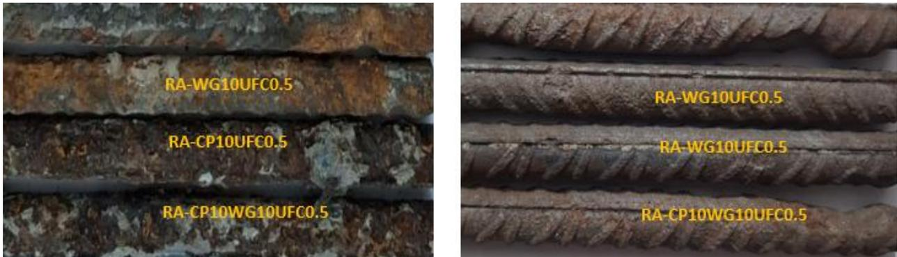
**Figure 4:** (a) Rebars before sandblasting, (b) The rebars after sandblasting.
