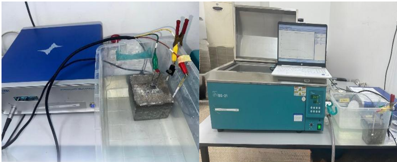
Figure 2. Electrochemical measurements using a three-electrode cell.
