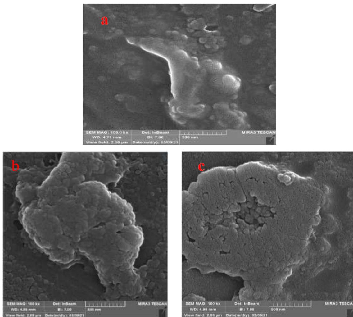
**Figure 6:** FE-SEM micrographs of TiO<sub>2</sub>NPs synthesised with laser energy of (a) 80 mJ, (b) 120mJ, and (c) 160mJ at 100 pulses.
