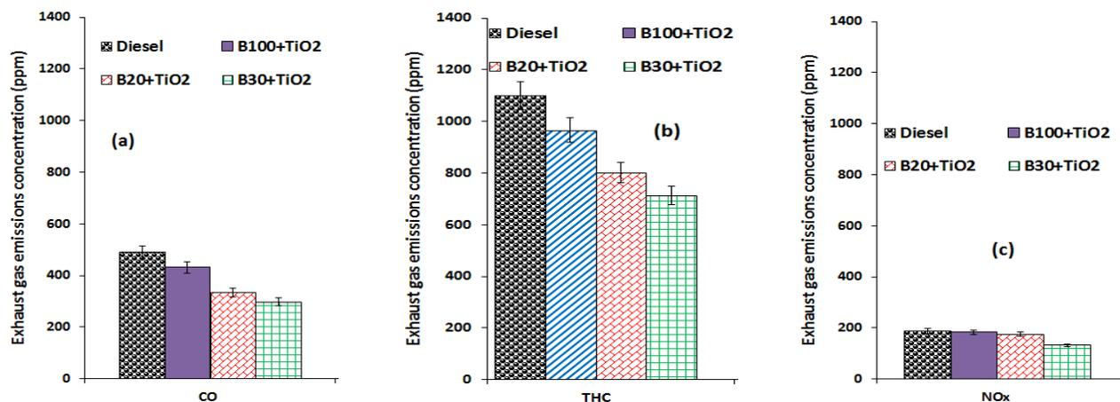
**Figure 2:** Exhaust gas emissions analysis of (a) CO, (b) THC and (c)  $\text{NO}_x$  for B100+ $\text{TiO}_2$ , B20+ $\text{TiO}_2$ , B30+ $\text{TiO}_2$  and diesel
