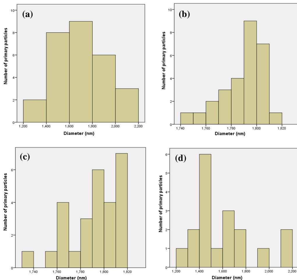
**Figure 5:** Number of soot particles for (a) diesel, (b) B100+TiO<sub>2</sub>, (c) B20+TiO<sub>2</sub> and (d) B30+TiO<sub>2</sub>
