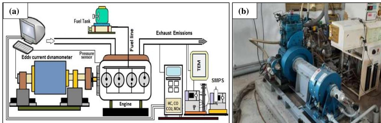
**Figure 1:** Research engine setup and tools for (a) schematic diagram and (b) real image of the research engine.
