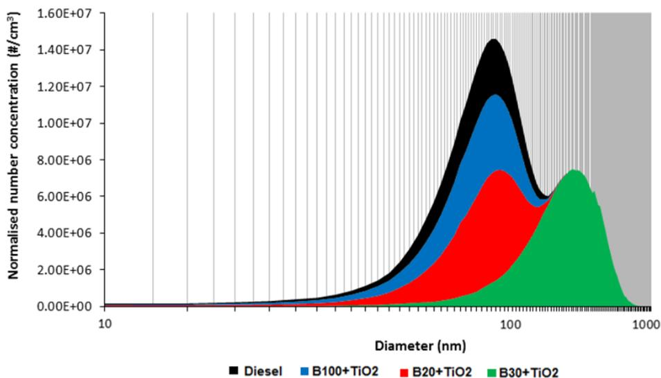
**Figure 3:** PM concentration and number for B100+TiO<sub>2</sub>, B20+TiO<sub>2</sub>, B30+TiO<sub>2</sub> and diesel
