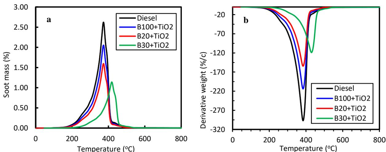
**Figure 4:** a) TGA analysis of soot mass for B100+TiO<sub>2</sub>, B20+TiO<sub>2</sub>, B30+TiO<sub>2</sub> and diesel. b) TGA analysis of soot weight for B100+TiO<sub>2</sub>, B20+TiO<sub>2</sub>, B30+TiO<sub>2</sub> and diesel.
